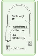
• Capacitance : 75pF/m Insulation resistance :  $1000 M\Omega$  Operating temperature : -20 to +110°C range · Cable outer : ø4.2mm : FEP/PUR(Black) diameter Material Waterproofing : NBR rubber cover · Sensor connector : TNC C02 (BNC) · Amp connector · Cable length : 5m
