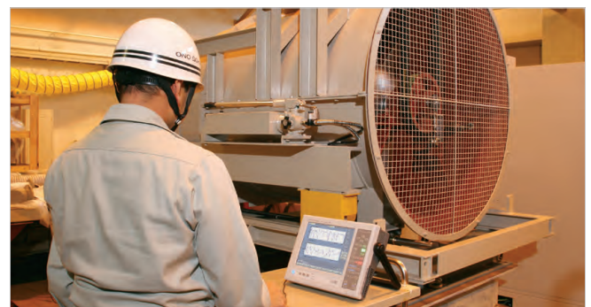
Rotational vibration measurement of a large blower using the CF-7200A
