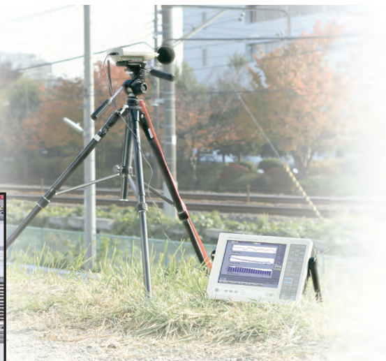
Outdoor noise analysis using the CF-7200A and the LA Series Sound Level Meter
