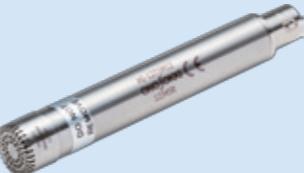
A microphone with a built-in amplifier. This microphone can be directly connected to a device equipped with a CCLD (constant current drive) power supply using a BNC cable. When connected to a TEDS-compatible device, information such as sensitivity is automatically read, eliminating the need for complicated calibration work. Reliable measurement and time reduction are achieved.
