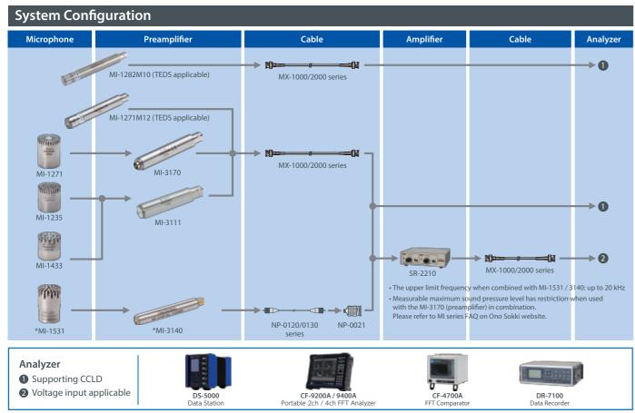
\*For measurements up to 100 kHz, CF-9200A / 9400A and DS-5000 100 kHz unit are recommended. CF-7200, DS-3000 and DS-2000 series 100 kHz unit (discontinued products) also can support
