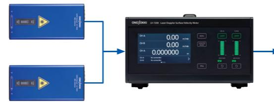
By connecting two sensors to one main unit, it enables to calculate and output difference in velocity/length between the two points. It measures the slip measurement between the roller and conveyed object in real time.
