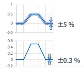
Up to four types of analog output (two types for each channel) can be selected from velocity, distance, velocity difference, and distance difference. Linearity: Max.  $\pm 0.3\%$  (LV-7100: Max. $\pm 5.0\%$ ) DC offset:  $\pm 0.3\%$  (LV-7100:  $\pm 5.0\%$ )
