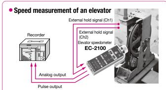
Make a measurement by pressing the circumferential ring to a pulley of governor or a rope. The instantaneous value is displayed by using the hold switch [1][2] on the main unit or using an external hold signal.
