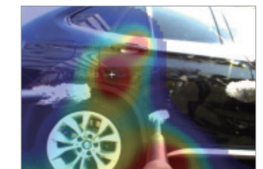
Synthesized sound of door hitting sound and ground reflection sound
