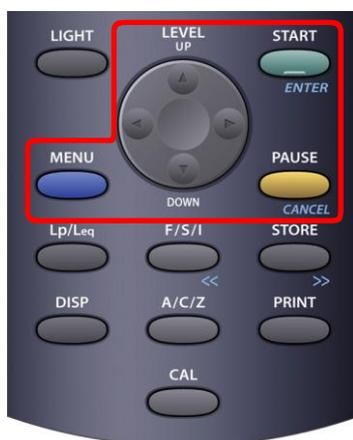
1. Press the “MENU” button on the measurement screen to display the menu. Press the [MENU] button while the menu is displayed, the screen is returned to the measurement screen.
