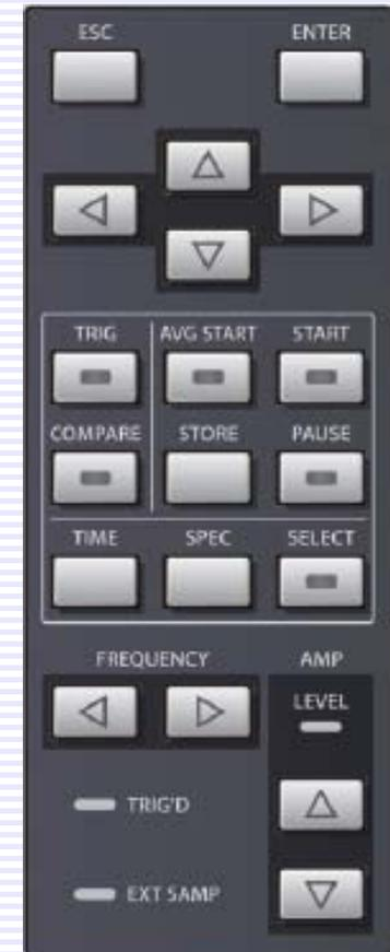
Set "SCHEDULE" to ON and press the START key on the panel. (In the example above, measurement lasts 40 seconds.)
