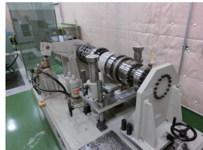
Durability testing with continuous load testing system
